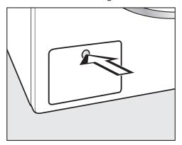
■ Press the drain pump access panel.
